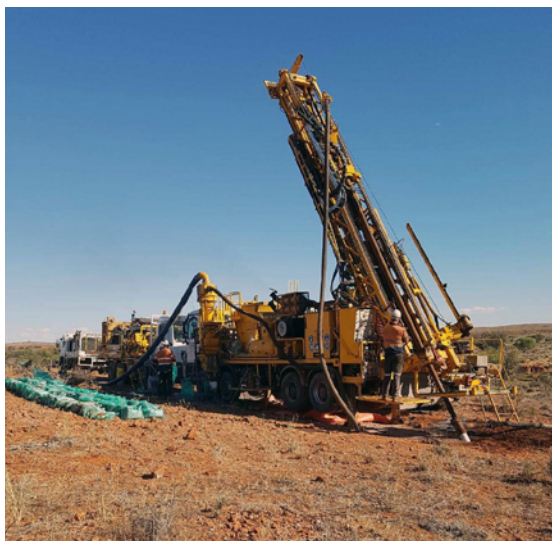
RC Drilling begins on site
