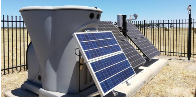
SODAR unit installed for 2022 pre-feasibility study into the establishment of a Renewables Energy Hub
