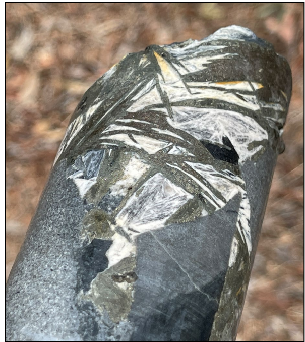
Figure 2. Spectacular bladed pyrite and sphalerite replacing or inter-grown with bladed wollastonite in brecciated sandstone fragments. Core is ØNQ. Depth of sample is 164m.
