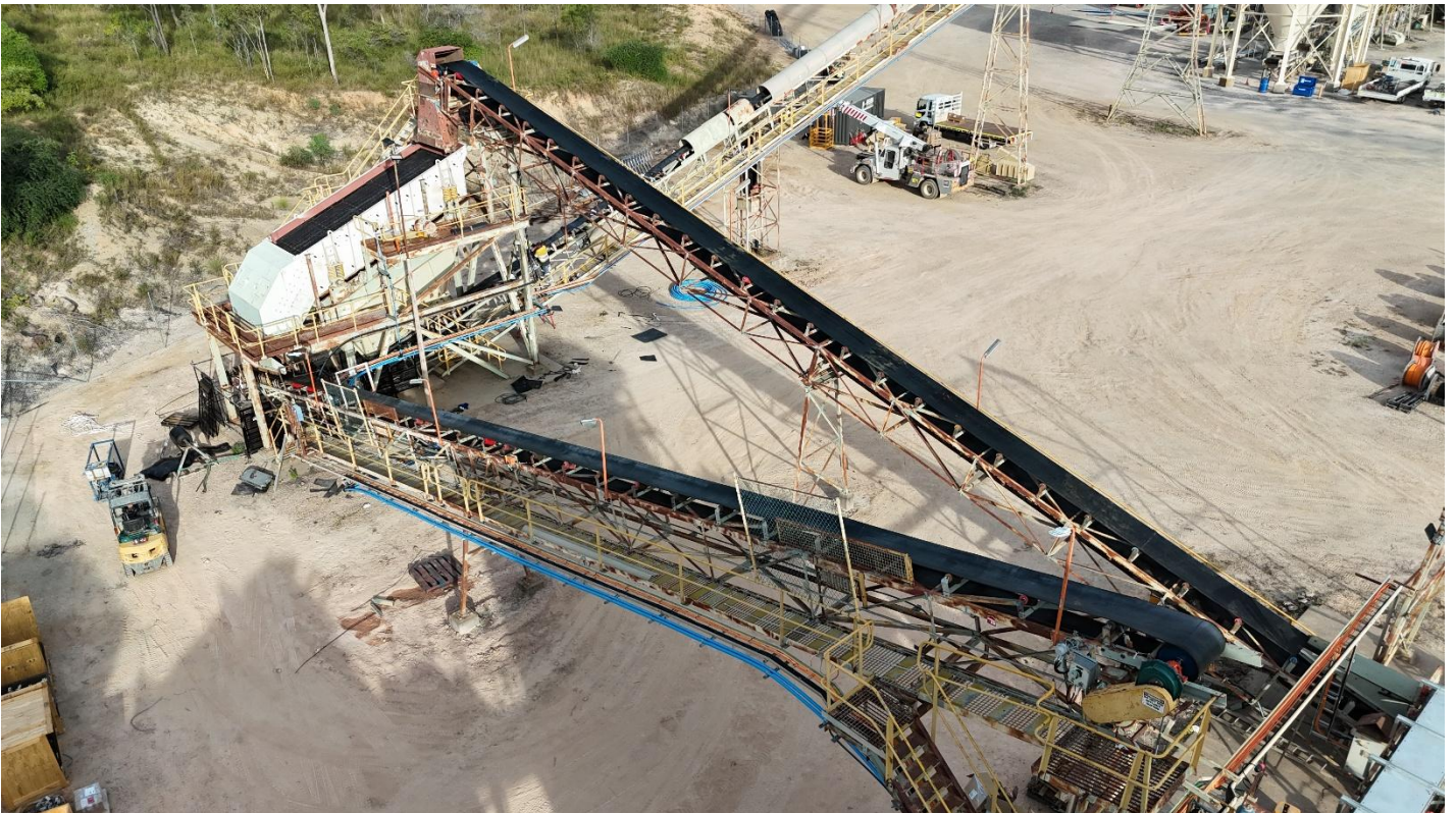
New belts installed for all five conveyors
