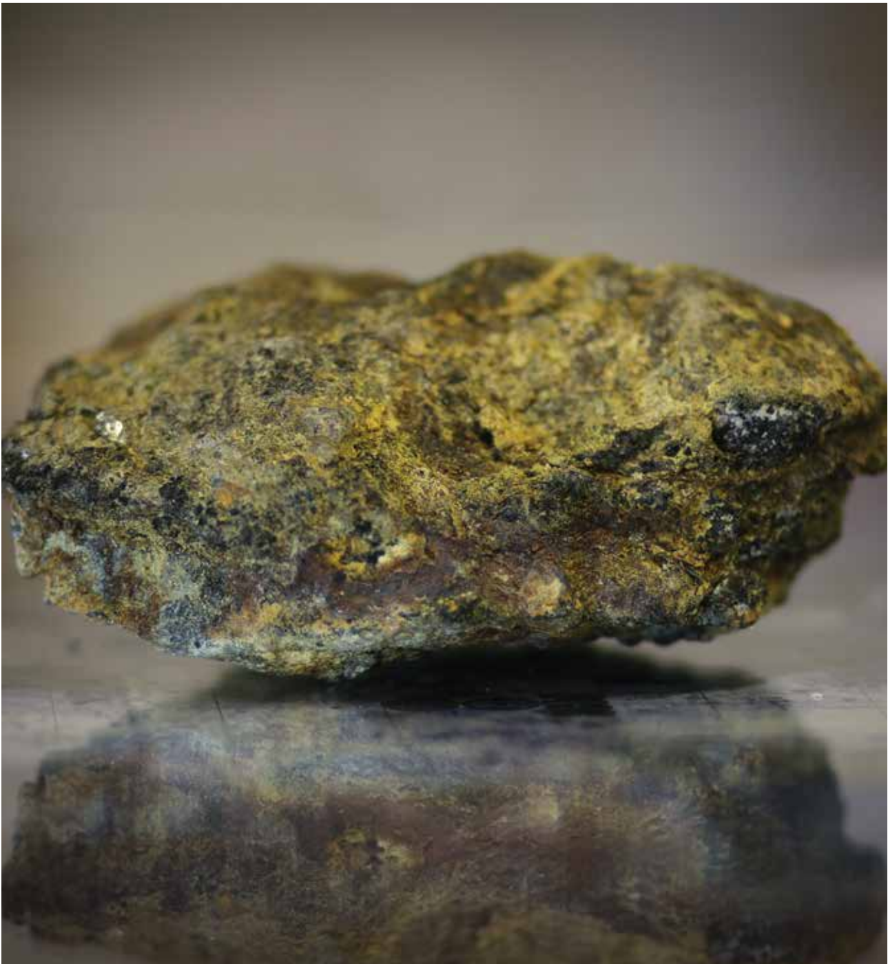
Oxidised lead and zinc mineralisation from the Prieska Project
