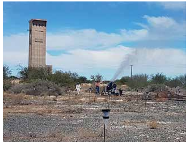
Feasibility study field trial of effectiveness of a 15kW evaporator at the Prieska Project. The planned pilot trials aim to test 75kW and 90kW units as the next phase of the program.
