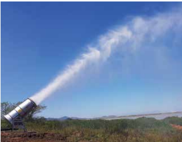
Feasibility study field trial of effectiveness of a 15kW evaporator at the Prieska Project. The planned pilot trials aim to test 75kW and 90kW units as the next phase of the program.
