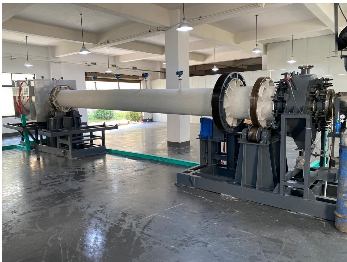
Image 1: Installation of pilot scale calcining unit at Hunan Firebird Battery Technologies' Plant
