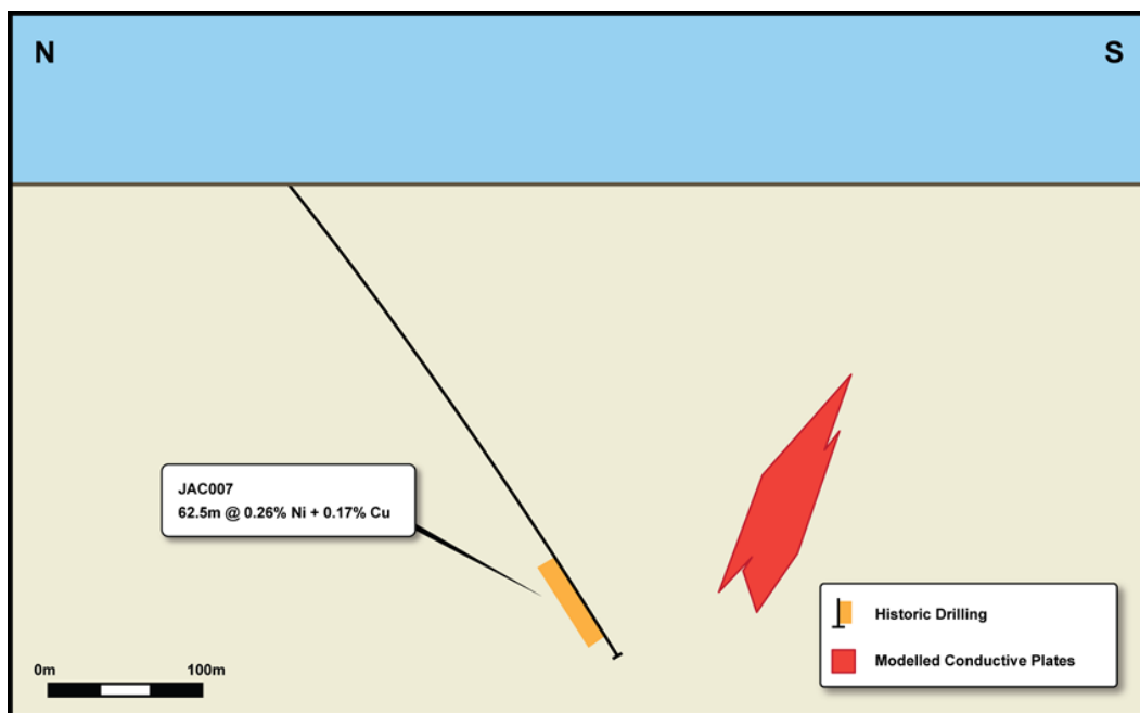
Figure 18: Section looking east through drill hole JAC007 showing the Ni-Cu sulphide intersection and newly detected FLTDEM conductors at Area 4.
