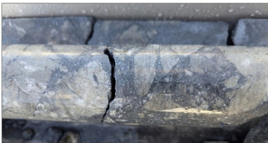
Figure 16: Core photo of the high-grade Sb interval in RDRC067 highlighting brecciated ultramafic at 239.4m. Refer ASX Release 26 August for full context)
