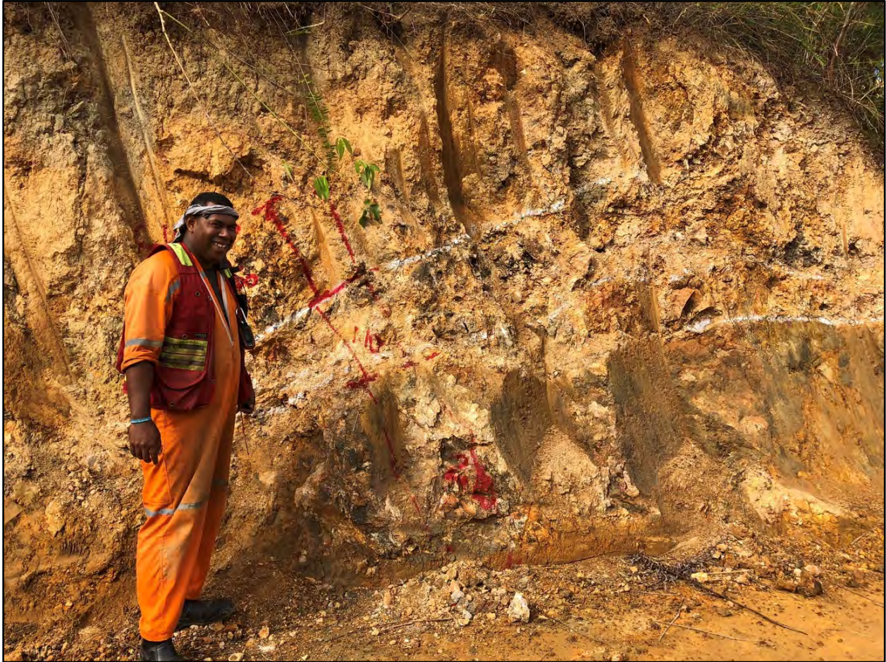
Figure 9-11: Example of chip channel sampling in a bench. The red marks indicate sample from and to locations, presented orthogonal to a structure (marked in white paint).
