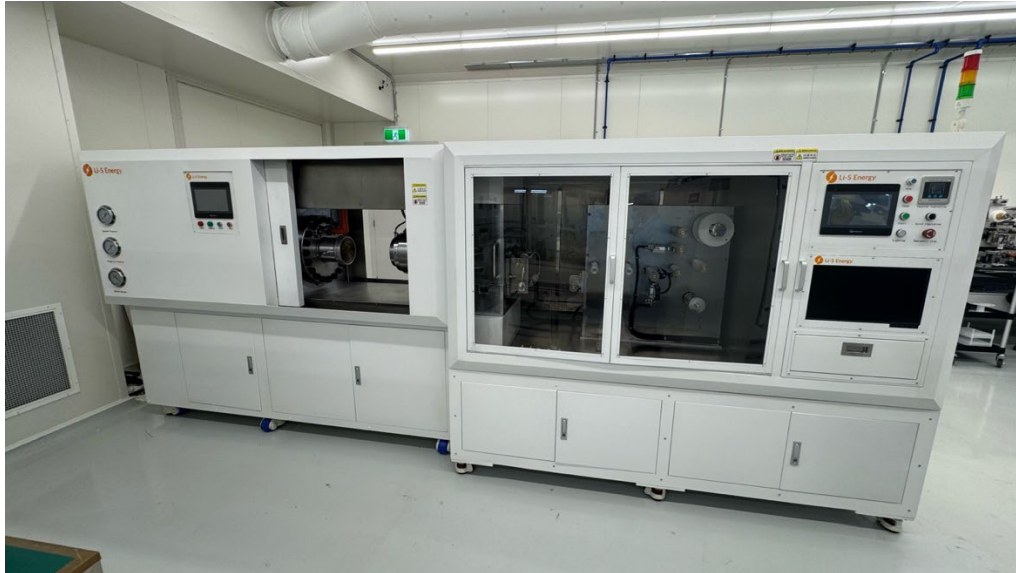
Image 2: Lithium Foil Extruder installed at Li-S' Phase 3 Facility in Geelong
