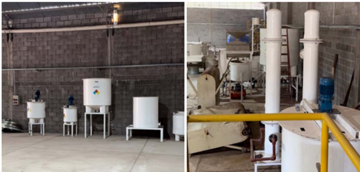
Figure 12: Plant mixing tanks and columns being refurbished at the new Pursuit Lithium Facility in Salta, Argentina
