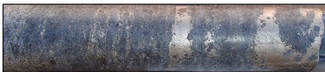
241m: zone with several Type 2 massive sulphide veins intruding the lithified pyroxenite along grain boundaries and stopping/entraining silicate autoliths. Note the metal fractionation to Cu-dominant margins.
