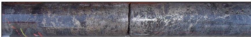
241m: zone with several Type 2 massive sulphide veins intruding the lithified pyroxenite along grain boundaries and stopping/entraining silicate autoliths. Note the metal fractionation to Cu-dominant margins.
