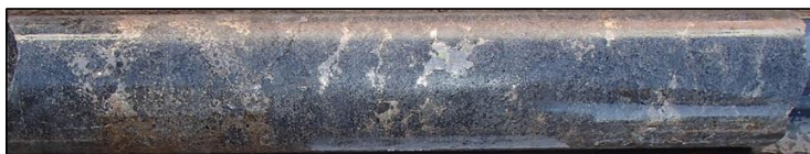
248m: 7m-thick zone with patchy and injected sulphide mineralisation causing incipient brecciation of the host norite. The sulphide mineralisation is polyminerallitic, hosting large grains of chalcopyrite derived from metal fractionation during sulphide liquid cooling.
