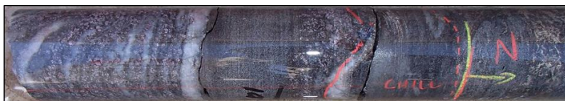
201m: Intrusion top contact, upper chill sharply cross-cut by a sulphide-mineralised pyroxenite magmatic breccia.
