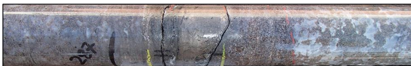
Figure 1: Drill hole OROD001 Ni-Cu sulphide intersections and brief descriptions. The mineralisation is typical primary immiscible magmatic sulphide derived under magma conduit conditions. No post-emplacement deformation is identified.
