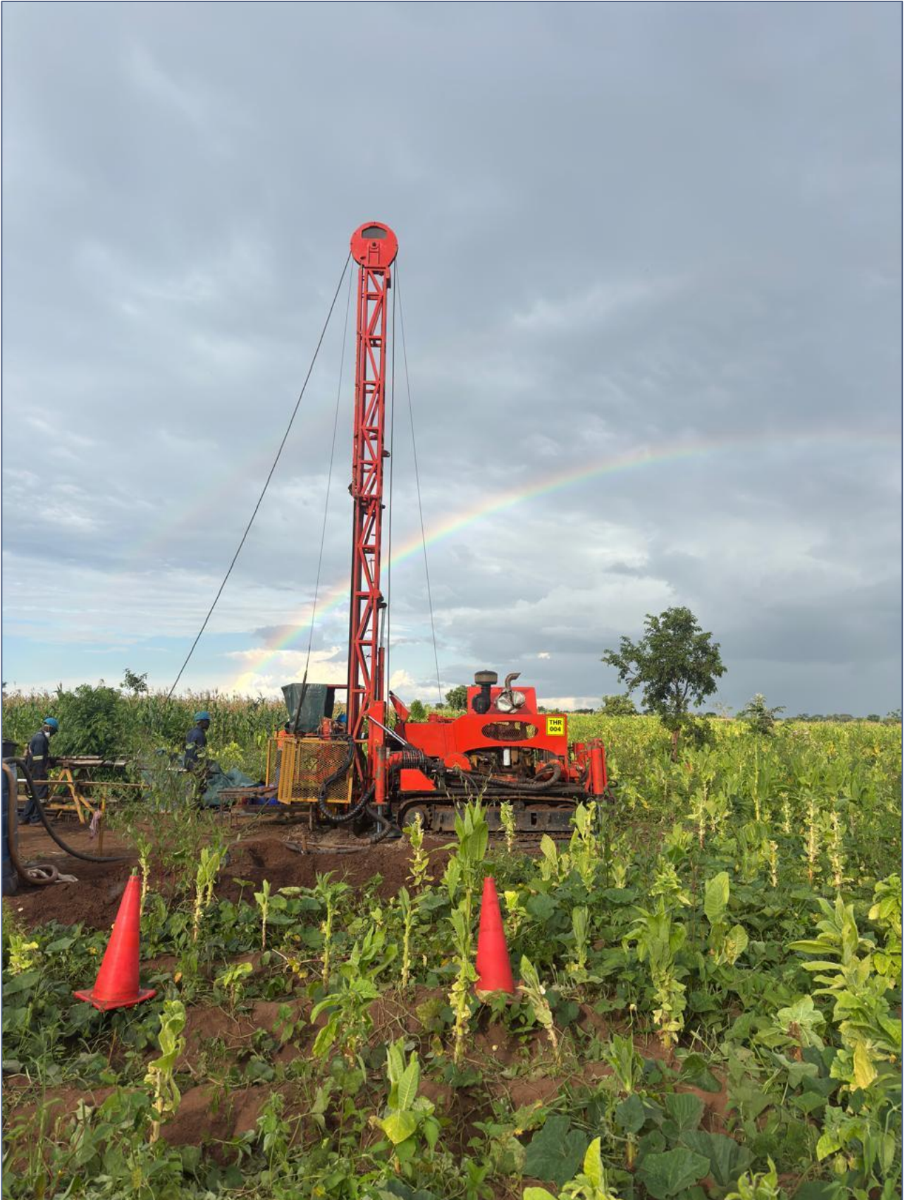
Figure 4: Geotechnical diamond drilling
