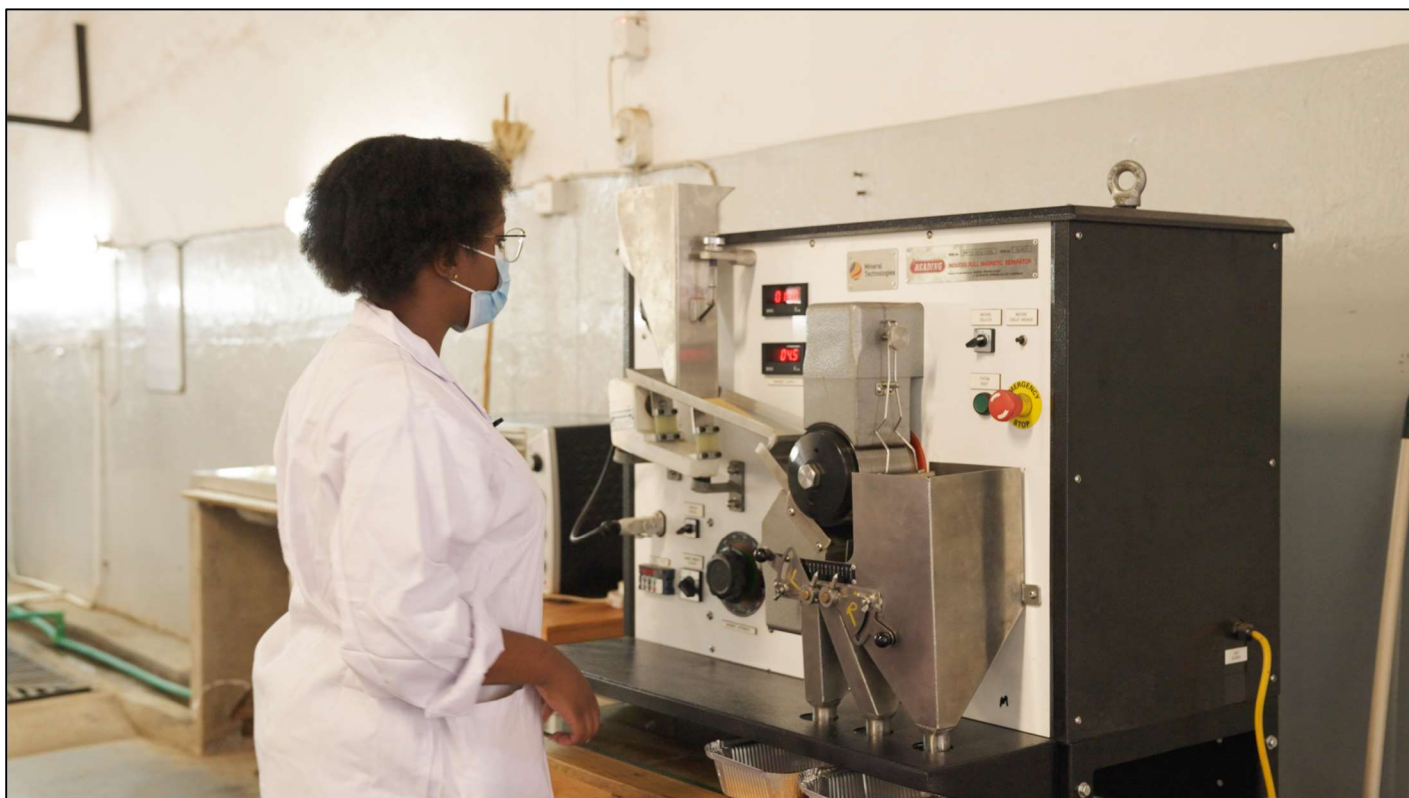
Figure 4: Bench-scale magnetic separator at Sovereign's Lilongwe facility separating non-magnetic rutile from other conductive minerals
