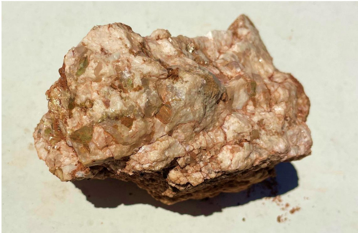
Figure 6: Fractionated pegmatite from Carr Boyd East containing Albite (70%) + Quartz (25%) + Rb Muscovite (5%) and Zinnwaldite (trace %). 7
