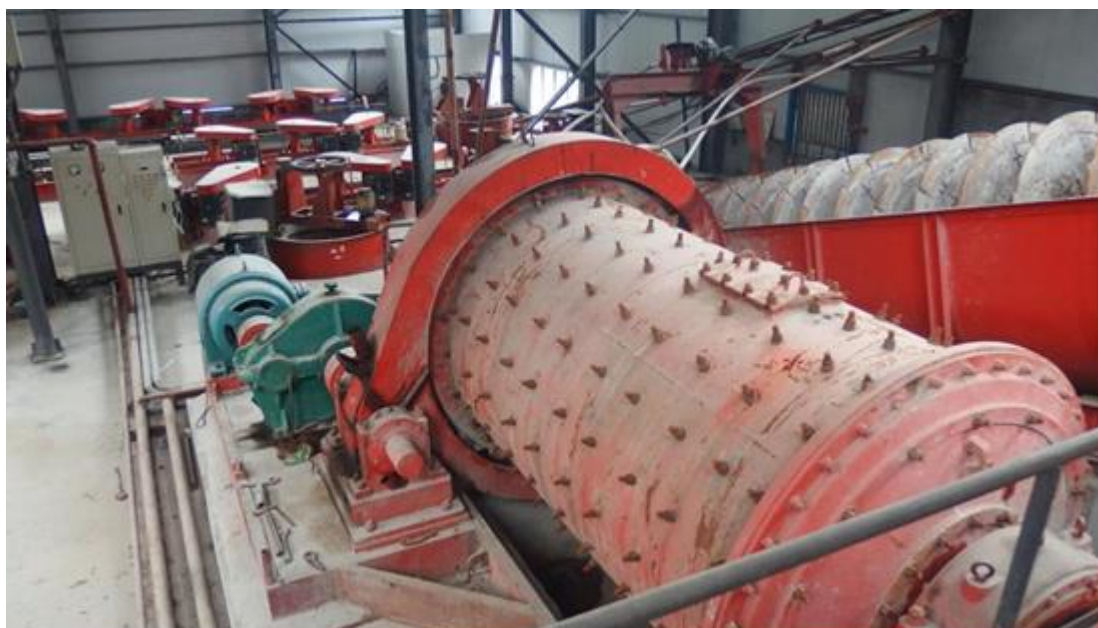
Figure 4-7 Ball mill crusher and floatation circuit.
