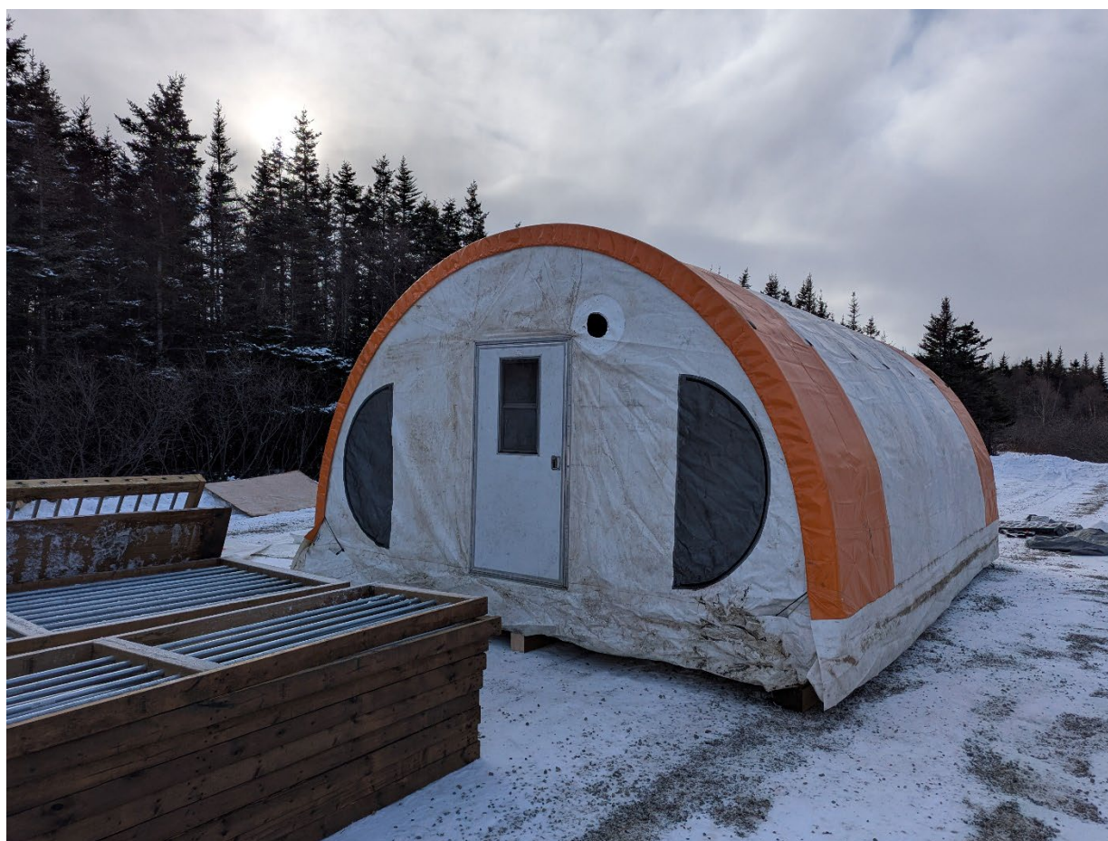
Figure 3: One of the core logging tents set up for use when the diamond drilling campaign commences. Storage and handling trays are in the foreground with snow on site already visible and temperatures averaging -2°C.
