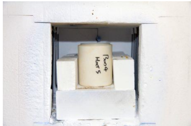
Figure 5: Positioning of magnesite sample in furnace
