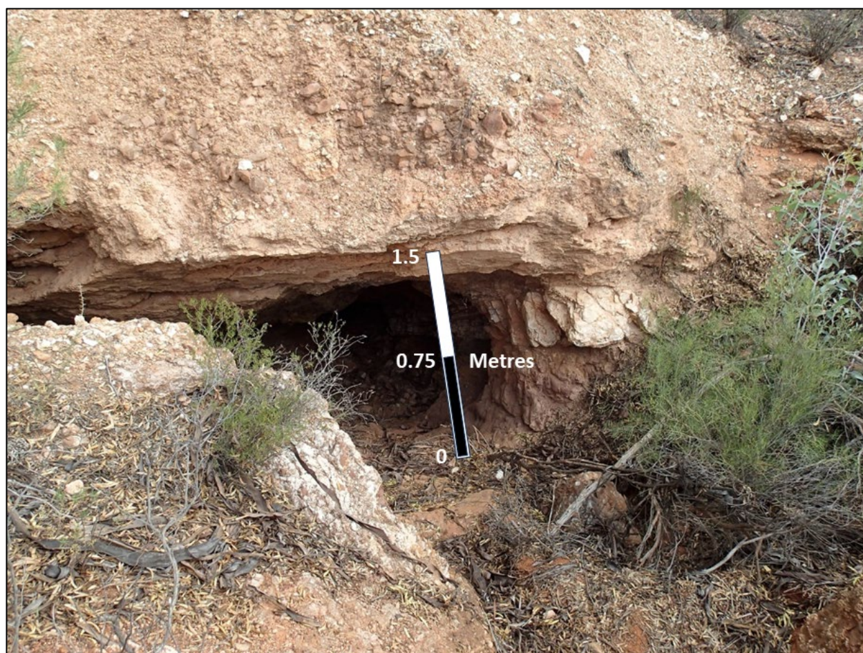
Figure 10: Cooe 1920s surface workings on south dipping quartz structure.
