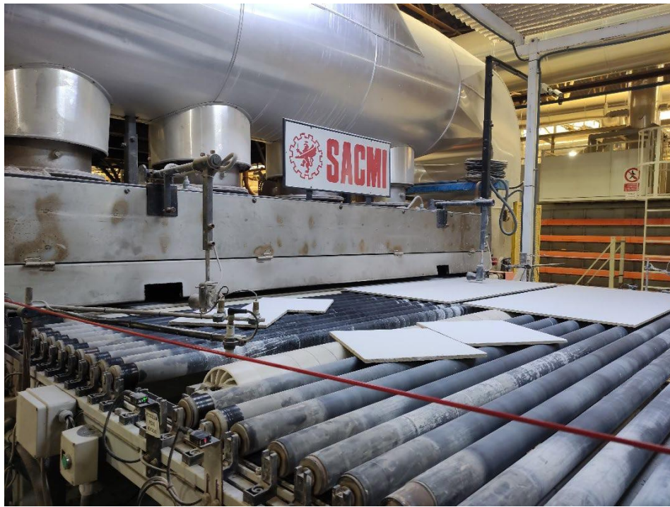
Figure 2 - Test tiles fired in an industrial kiln (Source: Pamesa)
