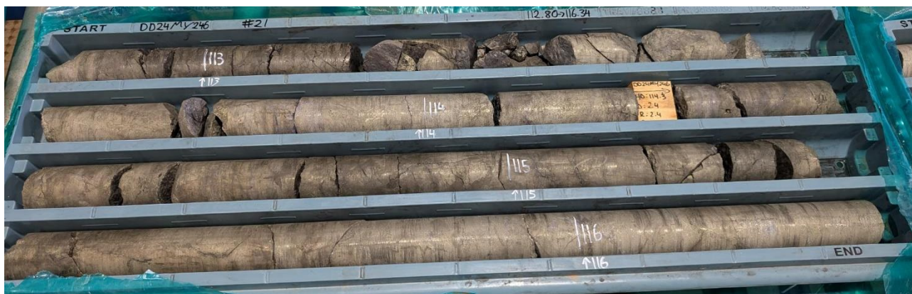
Figure 1: DD24MY246: massive pyrite-chalcopyrite -galena mineralisation approximately 113m downhole
