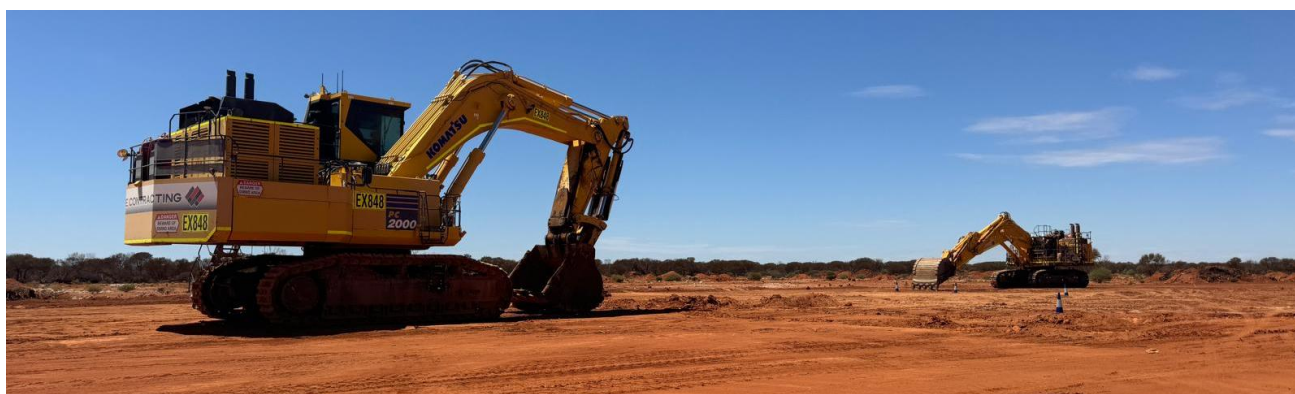
Figure 1: The 200t excavator and 125t excavator positioned at St Anne's north following commissioning, February 2025.
