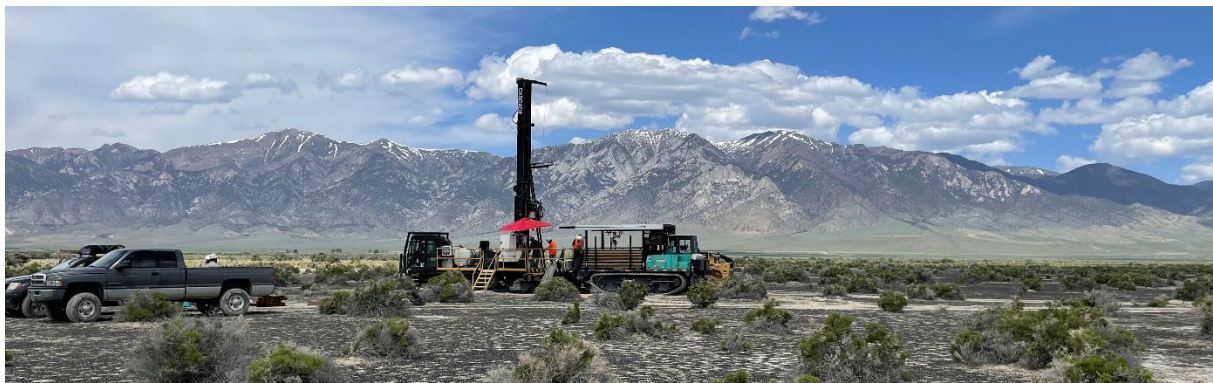
Figure 4: Sonic rig drilling at DH1
