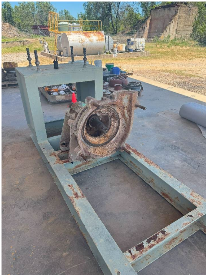
Area 02 Refurbishment of Warman cyclone feed pumps 01 and 02
