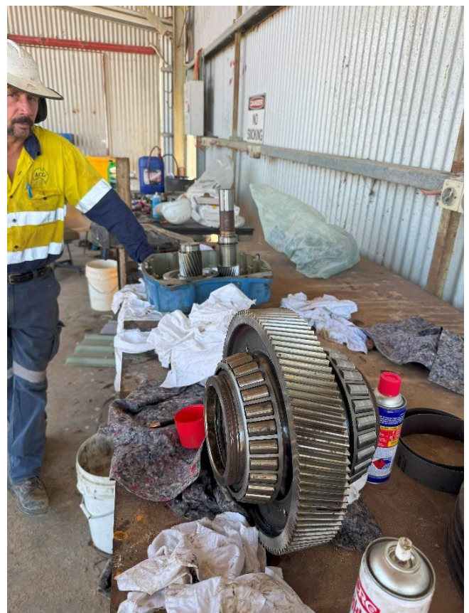
Area 01 Gear box removal and internal inspection of CV02
