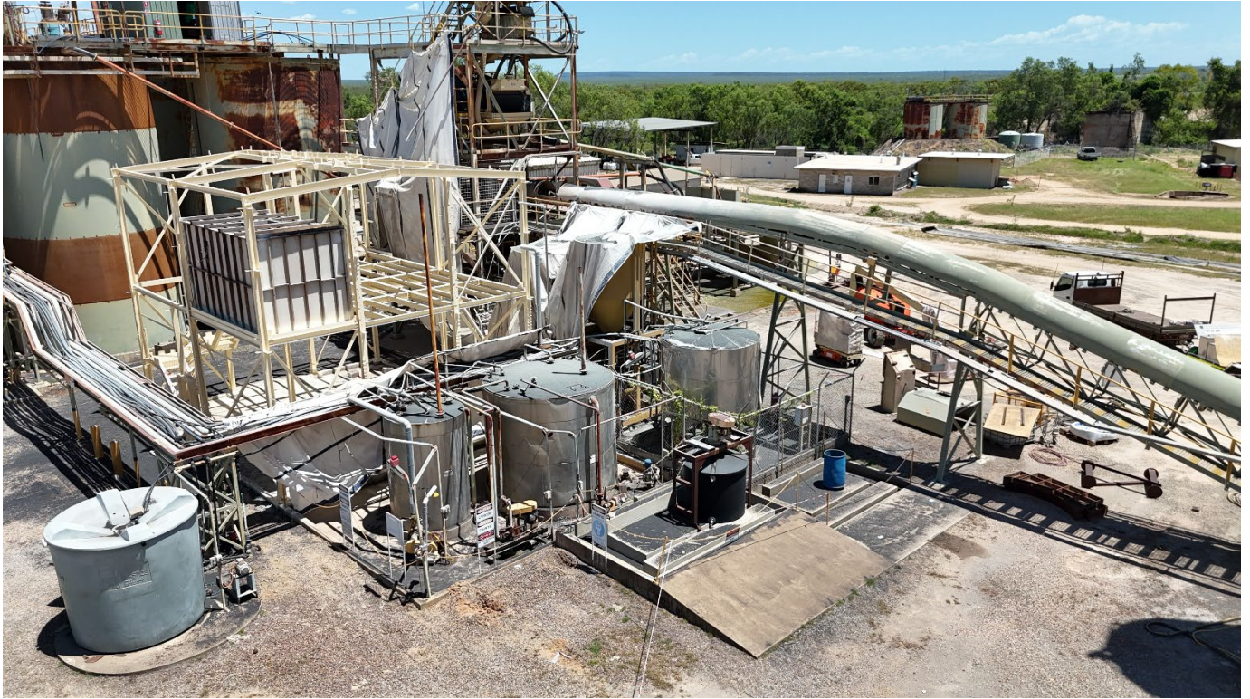
Final coated gold room main structure and work at 01-CV-06 Ball Mill Feed Conveyor
