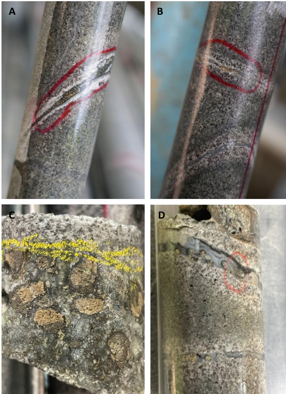
Figure 3. A) Coarse disseminated gold in a quartz-roscoelite veinlet, TGC-0034 67.5m. Sample returned 1396.3 g/t Au over 0.3m. B) Coarse gold in gray quartz veinlet, TGC-0034 81.6m. Sample returned 166.2 g/t Au over 0.9m. C) Coarse honey sphalerite rimmed by dark pyrite in variable light to dark gray quartz vein, TGC-0032 71.0m. Sample returned 112.9 g/t Au over 0.3m. D) Banded chalcidonic quartz-roscoelite-pyrite-fine native gold, TGC-0002 77.4m. Sample returned 44.3 g/t Au over 0.3m.
