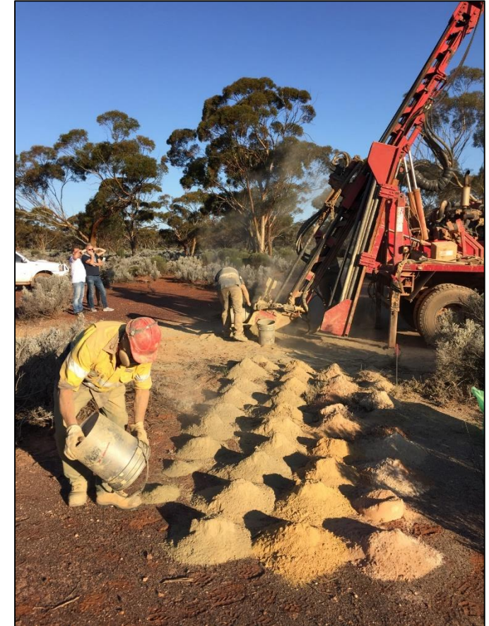
RAB Drilling at Torian's Zuleika JV Project.
