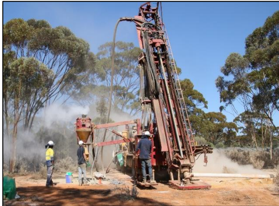
RC Drilling at Torian's Zuleika JV Project.
