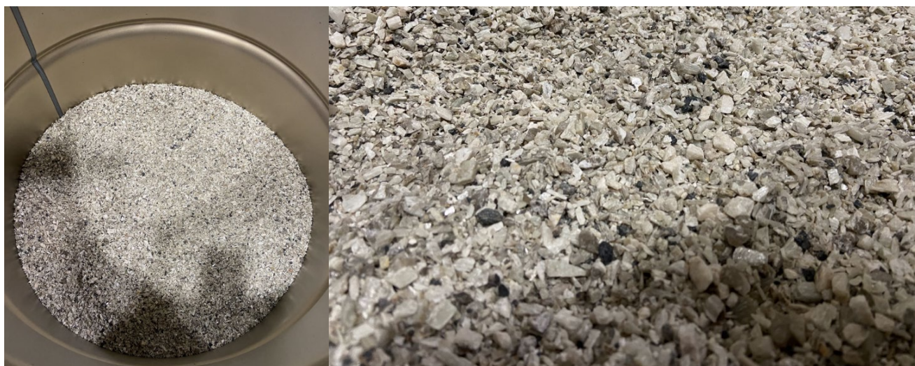
Figure 4: Spodumene Concentrate shipped to EcoPro's Korean Laboratory
