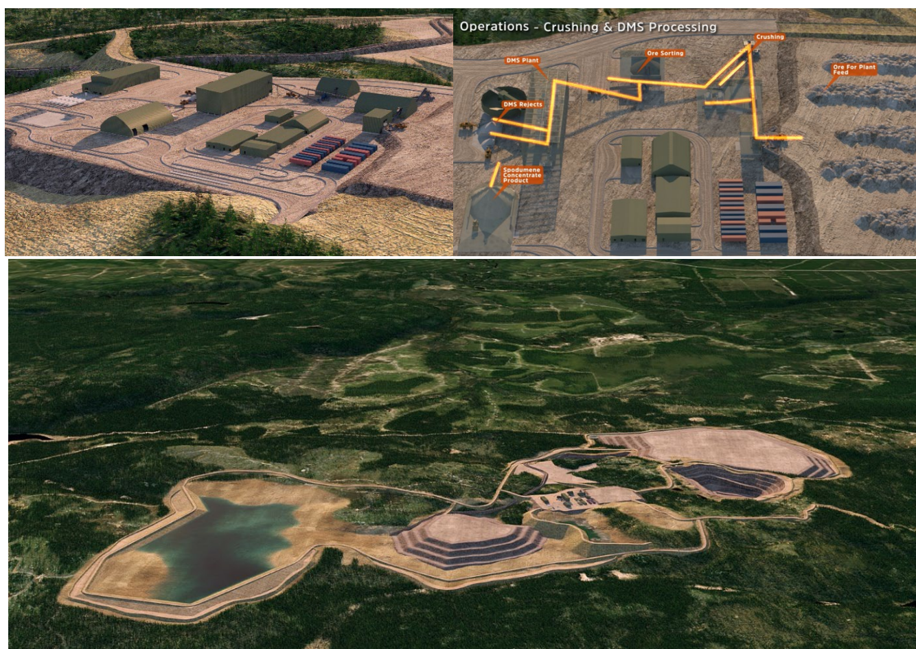
Figure 1: Rendered Seymour Project layout model showing views of processing plant, mining, and water management infrastructure
