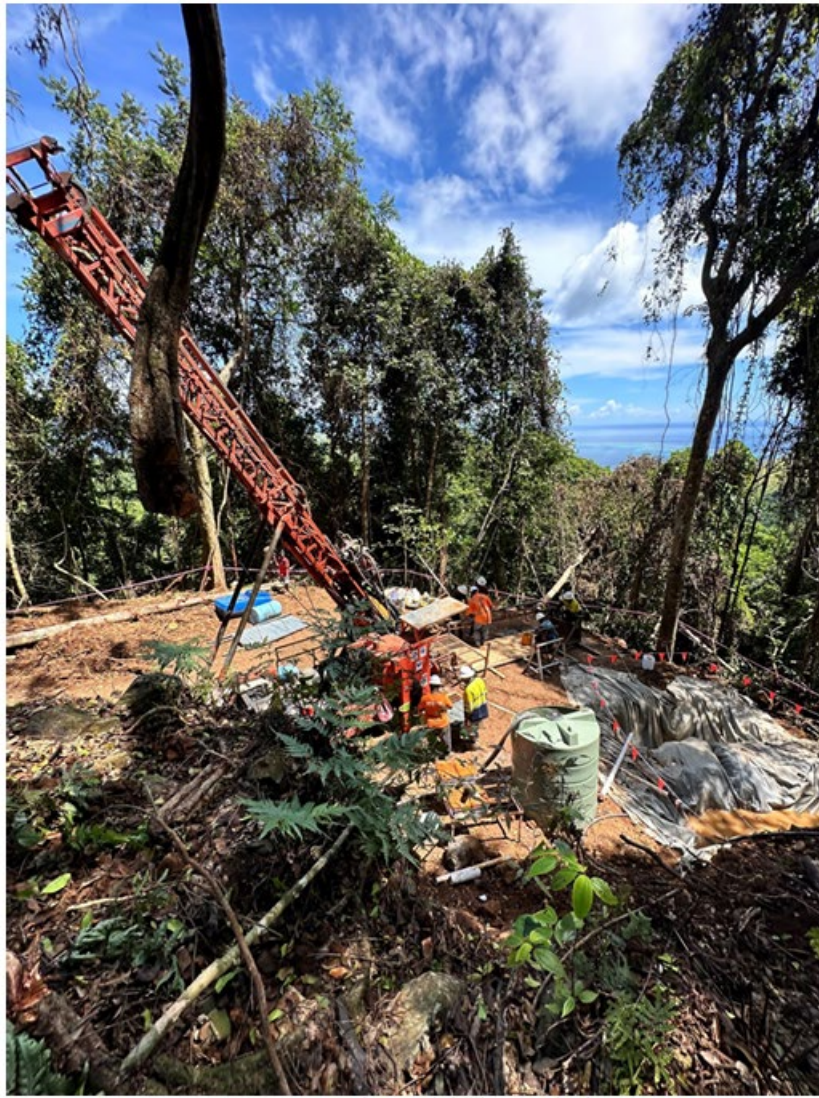
Figure 4 – Diamond drilling at Viani
