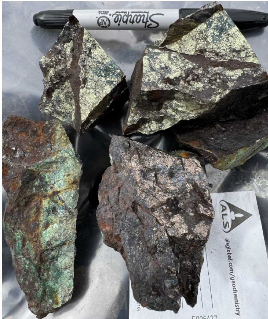
Figure 1 – Rock Sample F005437 from a mineralised outcrop of massive chalcopyrite-bornite at the Glacier IOCG Target
