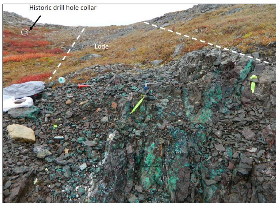
Figure 6 - Field photographs of the Cu-TAR mineralisation (Lode No. 2) taken by Tundra Copper Corp in 2014. Photo illustrates the 2.5 m continuous chip sample which returned 2.5m at 10.3% Cu and 5g/t Ag. (NUMIN File Reference 086024)
