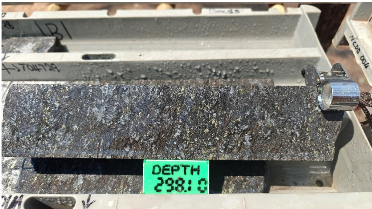
Figure 1. High grade copper mineralisation (as chalcopyrite) in Ore Schist unit from Nyungu Central (Hole NCDD004; core shown from downhole depth 298.1 metres)
