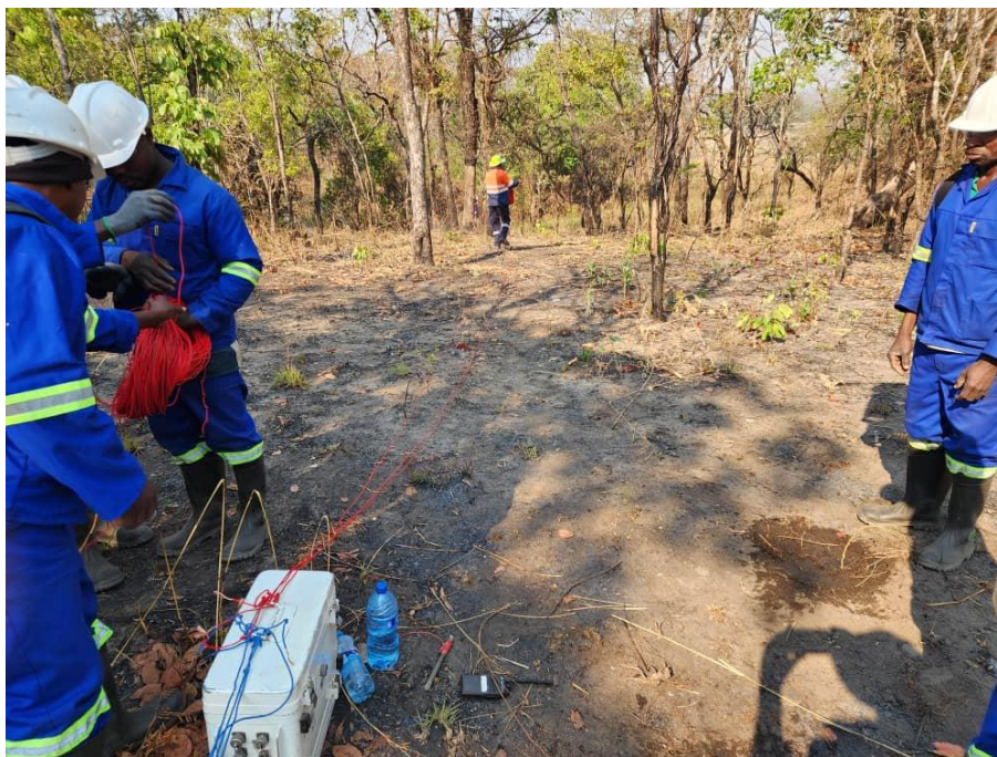
Figure 5: IP surveying underway at the Kapikuba Prospect
