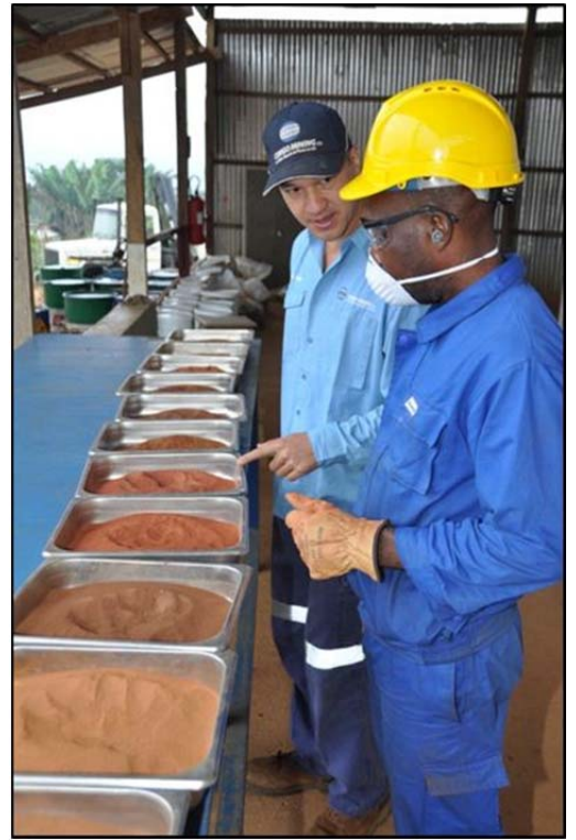
Figure 5: Preparation of trench samples at the Mayoko Sample Preparation Laboratory
