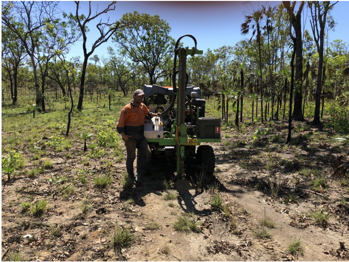
Figure 3 ATV-mounted auger used to map concealed pegmatites at Finnis through shallow soils near surface.
