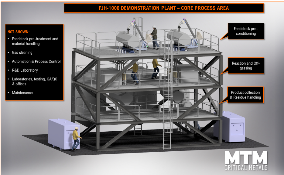
Fig 2. Conceptual artist’s impression of the Core Process Area of the FJH Demonstration Plant
