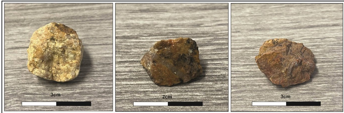
Figure 3: Bottom of hole rock chip samples GVAC025 – weakly altered granitoid (left), GVAC024 (middle) and GVAC023 (right) strong hematite-silica alteration.
