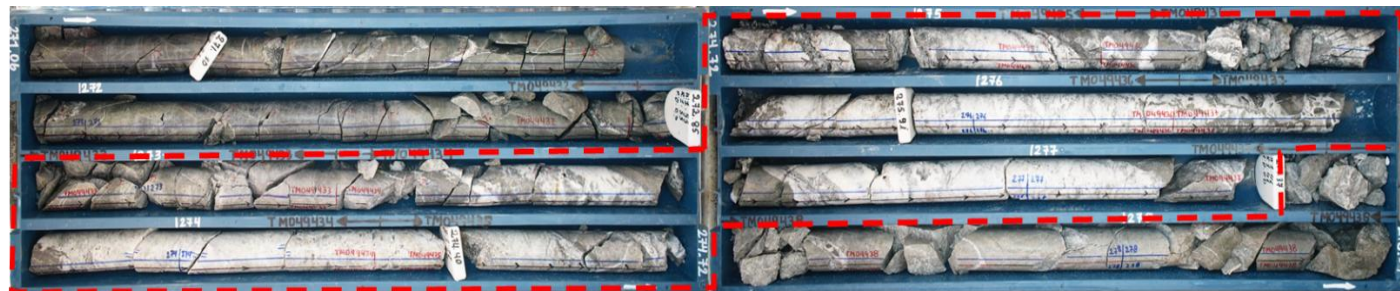
Plate 2. Drill core from CVDD24-120 mineralised zone, 4.1m @ 3.7 g/t Au, 8.7 g/t Ag from 273.2m)
