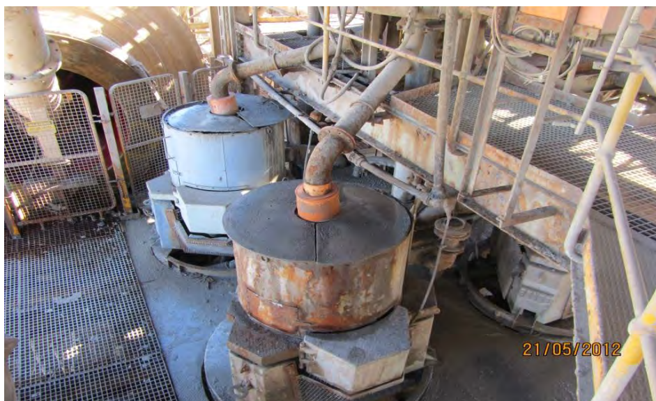
Figure 3.43 Knelson concentrators
