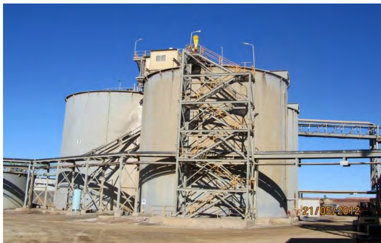
Figure 3.45 Cyanidation tanks
