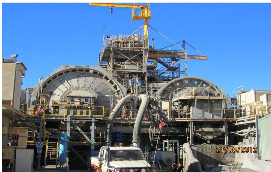
Figure 3.42 Ball and SAG mill
