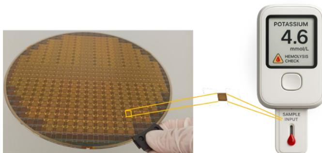
(Left) is a wafer full of Archer's biochips. (Right) is a conceptual drawing of our handheld reader with a sample cartridge inserted. The Biochip will be integrated into the cartridge where it receives the blood sample and measures the potassium levels in the blood.
