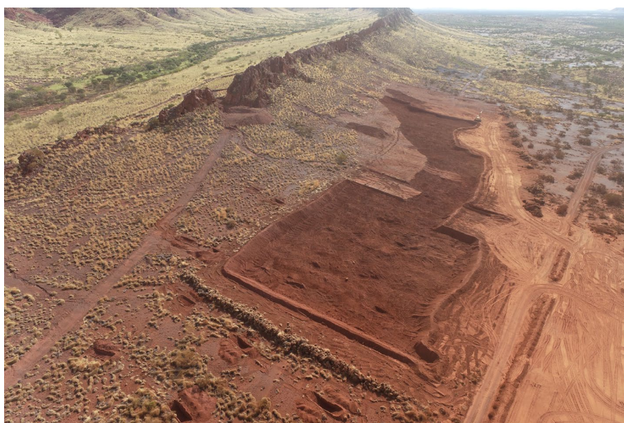
Figure 7: Excavation of Detritals Iron Ore on Northern Slope of Paulsens East Hematite Ridge
