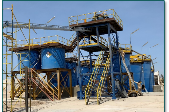
Figure 5 | CIP Circuit Installation complete and system tests in progress
