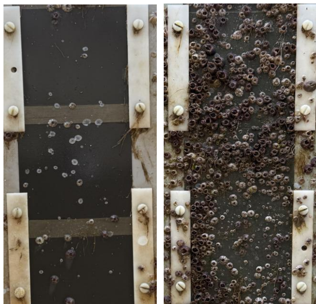
Figure 3: Field testing conducted within the ITTC; (left) graphene-enhanced coating (right) control coating after 10 weeks
