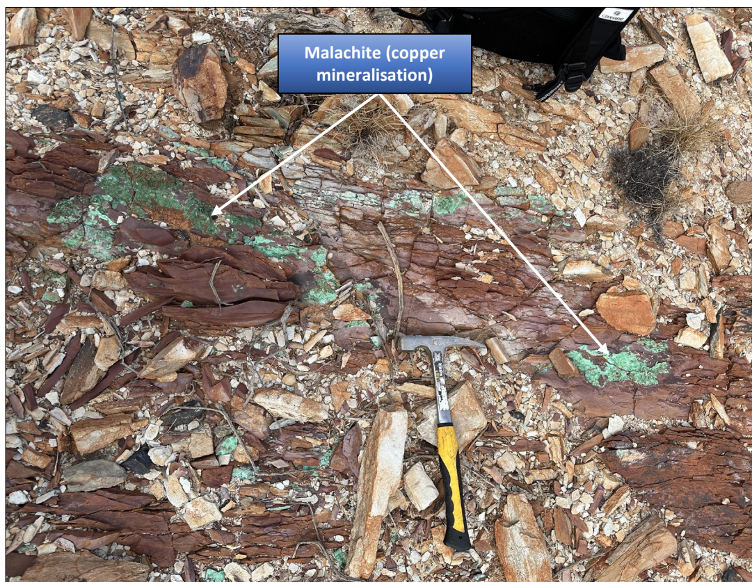
Figure 2 – Rock Chip Sample CH213 - Malachite eastern edge of 8-10m copper zone, strike 160° dip -30. Assay Results: 8.64% Cu
