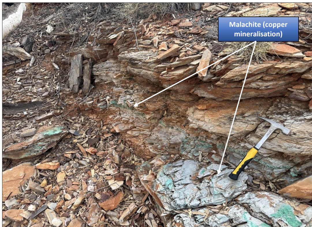
Figure 3 – Rock Chip Sample CH215 - Layered Malachite in creek bed, dipping 15° to west Assay Results: 13.95% Cu
