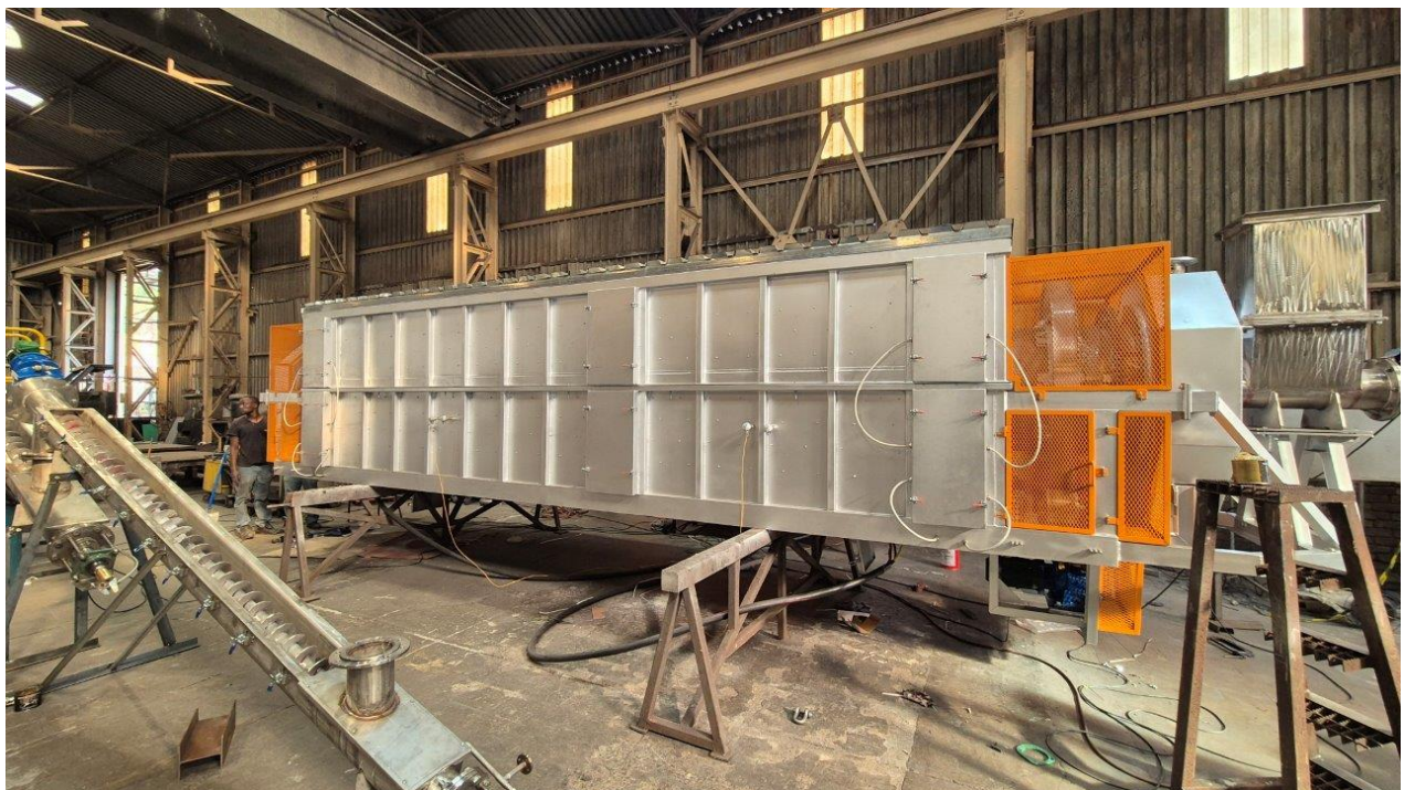
Figure 2: Calciner and screwfeeder
