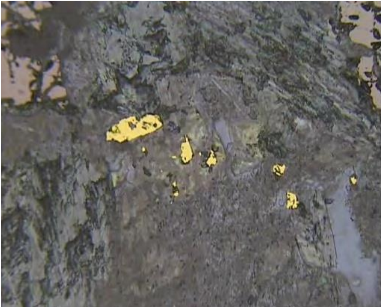
Figure 12: photomicrograph of sample 137002.20 from 1295.2 metres, showing fine grained chalcopyrite intergrown with pyrite and amphibole alteration after mafic mineral within alkaline gabbroic diorite.
