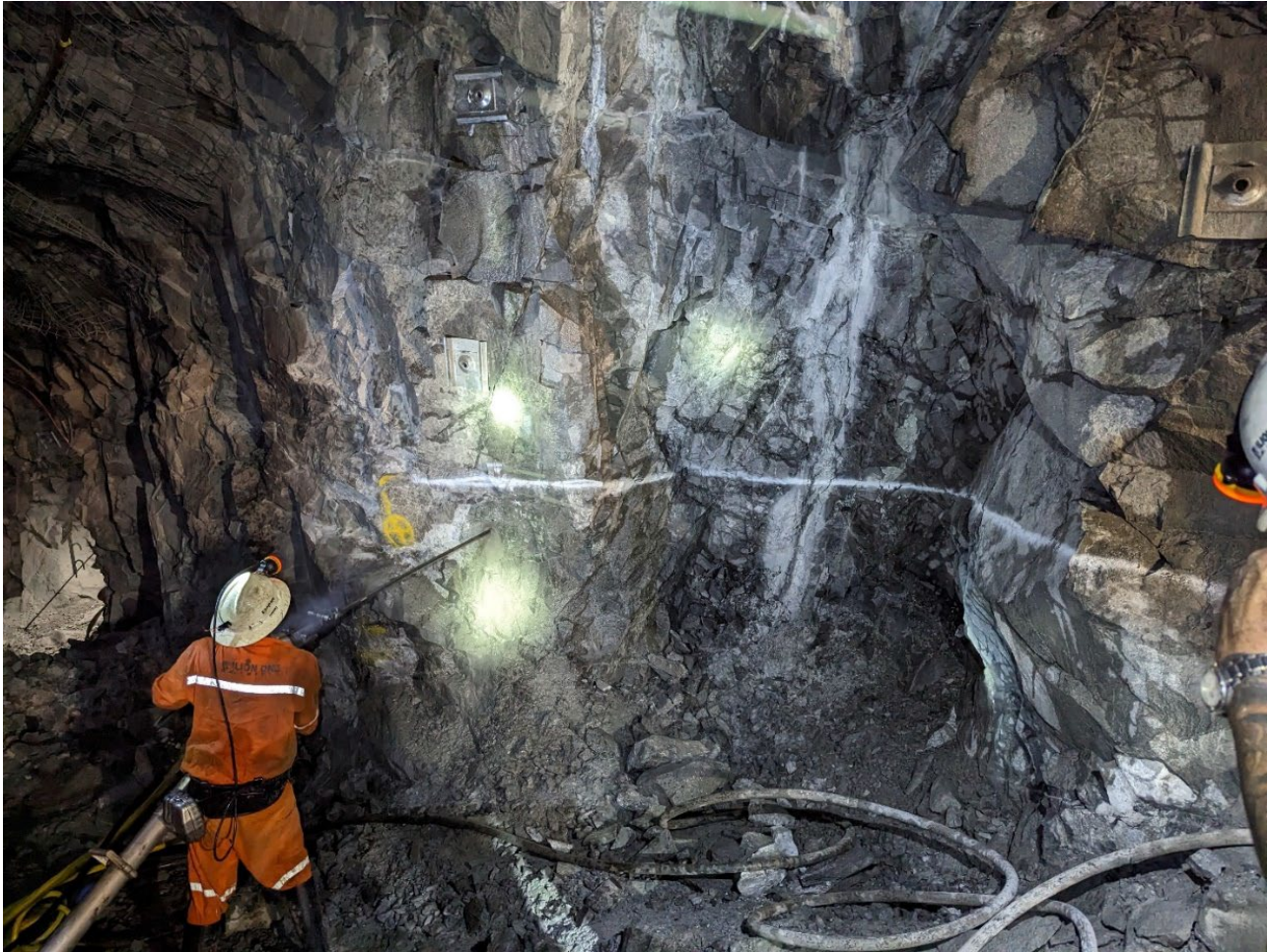
Figure 1. Photo of the first cut on the lode, strike drive from the new development decline.
