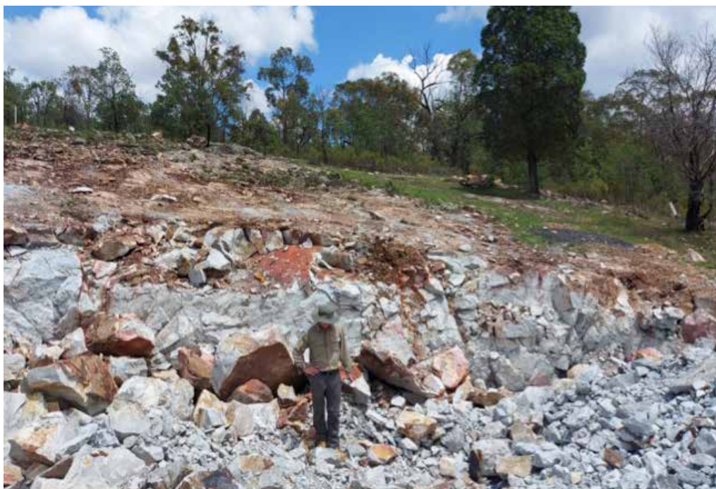
Figure 7: bulk sample blast site showing mineralised fractures.
