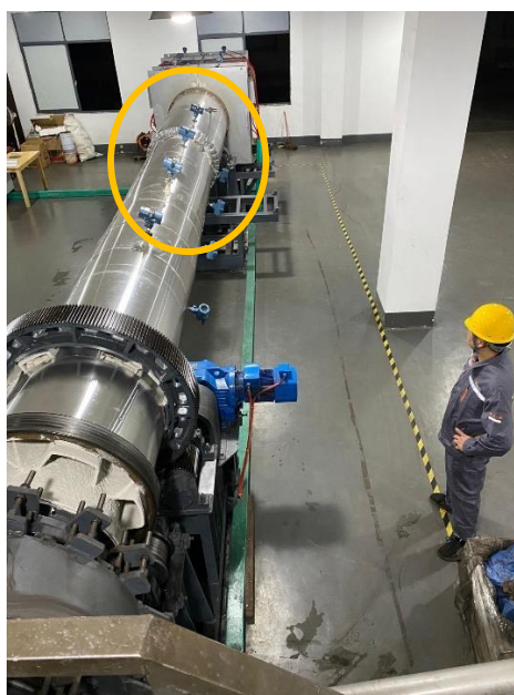
Image 2: Calcining Kiln with temperature gauges highlighted
