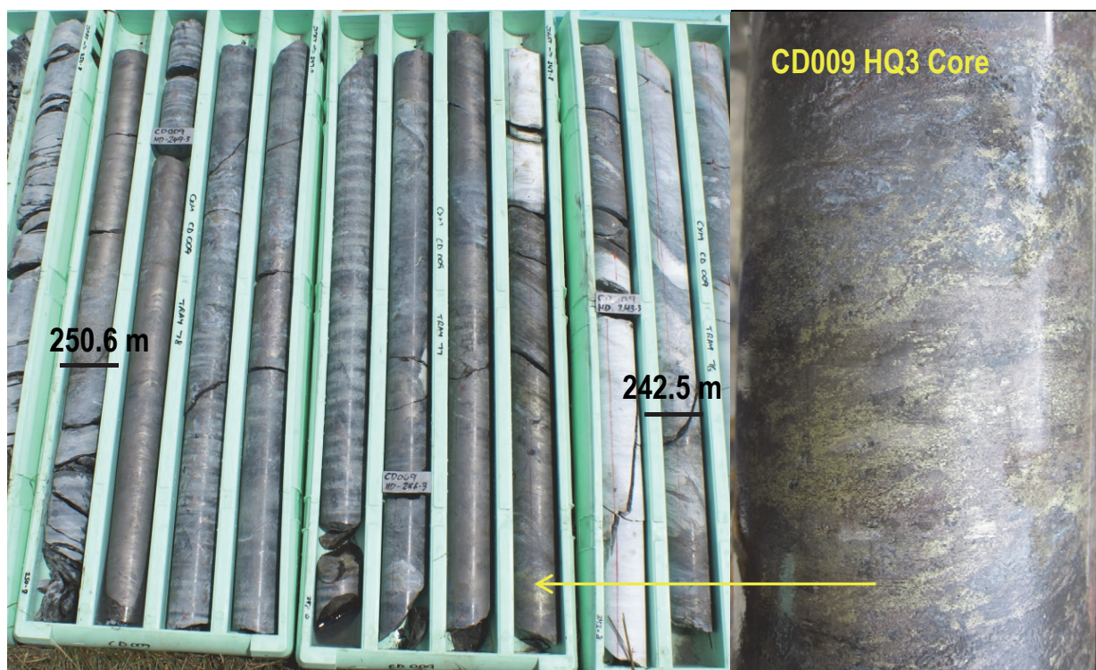
Figure: CD009 drill core with massive sulphides, marble and altered volcanics (242.5m to 250.6m).
