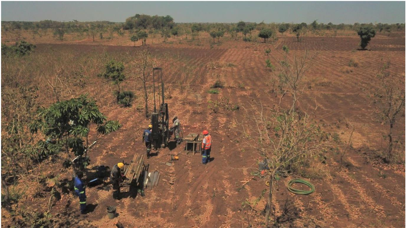
Figure 4: Drone photograph of the push-tube core rig in action at Kasiya.
