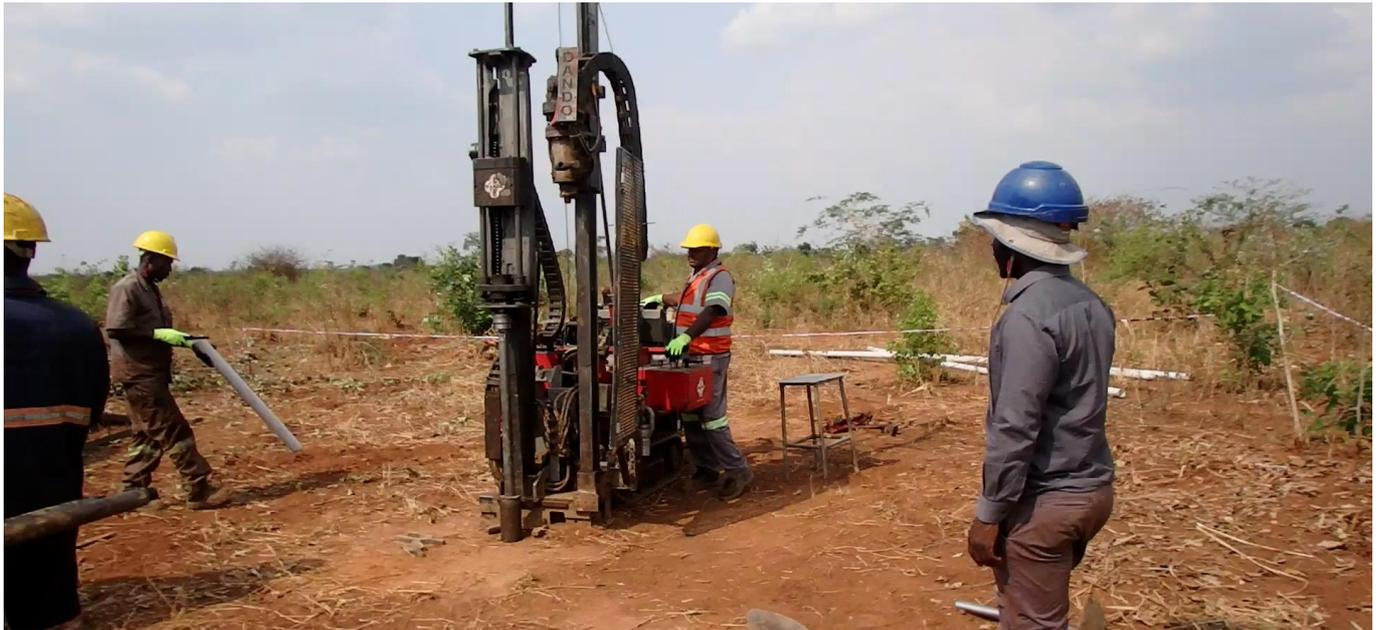
Figure 3. Push-tube core drilling at Kasiya.
