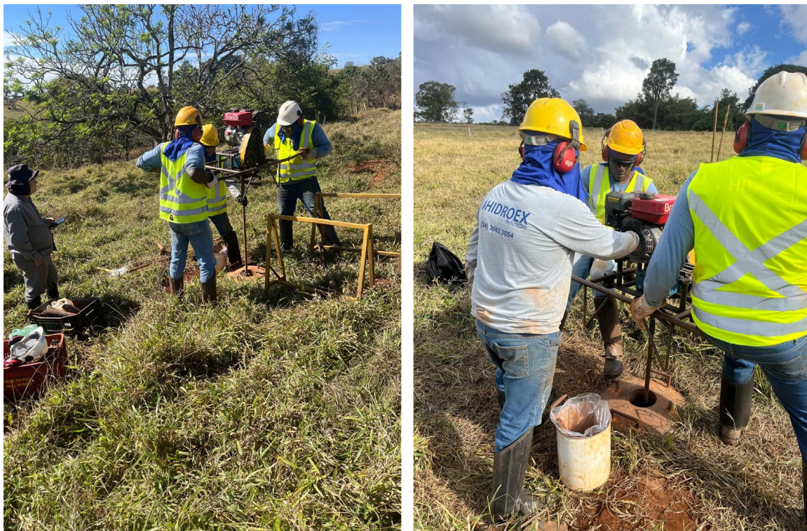
Figure 4 – Auger drilling underway at the Araxa Project.
